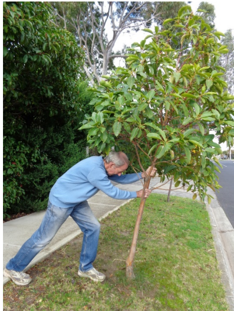
Figure 1. The Burnley test for investigating street tree stability and root development
