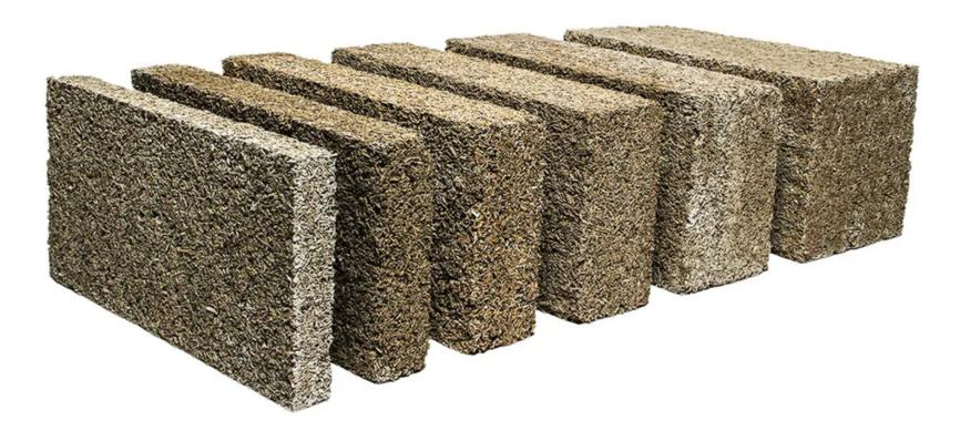
As mentioned above, Hempcrete is a biocomposite of hemp *hurd* or *shiv* together with lime. The mixture is prepared by combining the above components with suitable quantities of water. The lime acts as a binder that coats the hemp particles and, once it reacts with the water, the lime glues the hemp particles together to provide a high material strength. Any excess moisture is removed from the blend. The resultant residue is Hempcrete.
