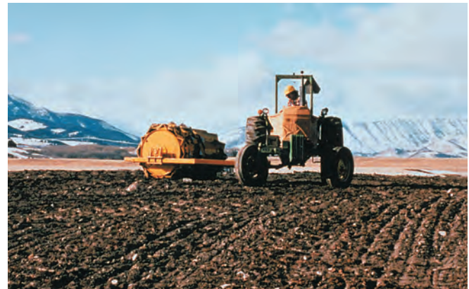
Imprinters, such as this Dixon land imprinter, leave a waffle-like impression as they pack soil.
