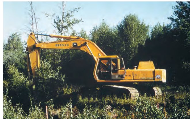
Backhoes are used to lift large plugs of native plant material. They are often used for aquatic plants.
