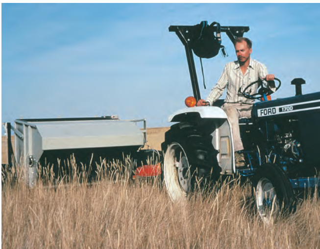
A seed stripper, pulled behind a tractor, is suitable for large, relatively uniform sites.
