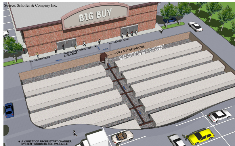
INFILTRATION CHAMBER SYSTEM UNDER A PARKING LOT
