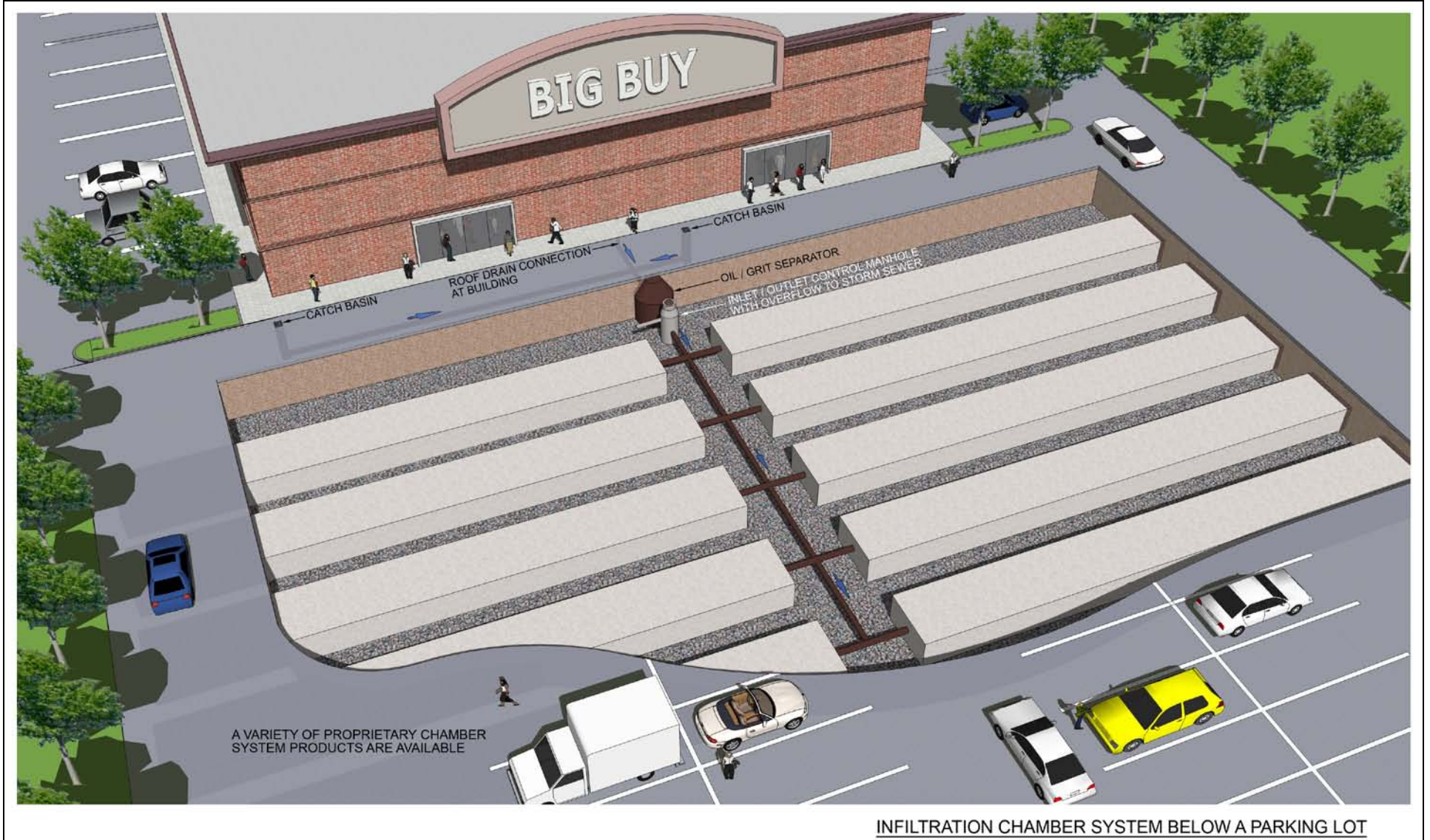
Figure 4.4.7 Schematic of an infiltration chamber system below a parking lot
