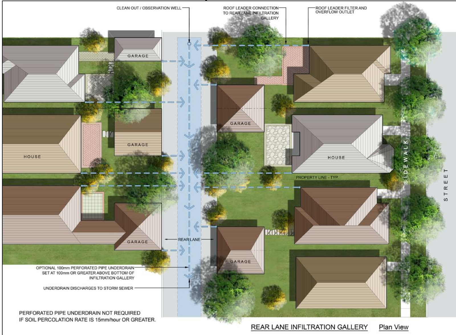
Figure 4.4.5 Plan view of an infiltration trench below a laneway
