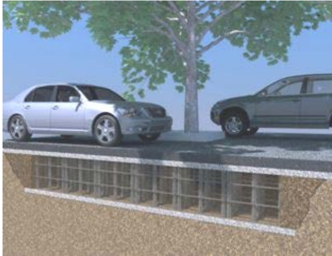
FIGURE G.3 — MODULAR CELL SYSTEMS (Source: [42] Greenmax, 2013.)
