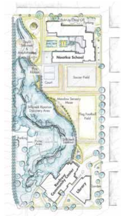
Revealing Still Creek Master Plan: To daylight Still Creek in the Nootka Elementary school yard, the sport courts/fields will be relocated to the south of the school, which, with the help of the long linear play ribbon, creates a greater programming and circulation connection between the school, park, and community center. All images courtesy of Mickella Sjoquist, Stephanie Aitken, Yiwen Ruan, Heather Scott.
