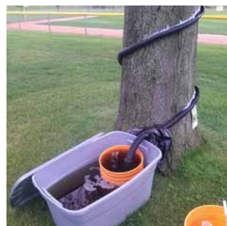
Figure 3 below. Stemflow collection system. Photo credit: Julie Schooling
